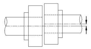
**7.7.3**- When installing the coupling, please observe the maximum permissible angular displacement.
