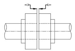
**7.7.2**- When installing the coupling, please observe the maximum permissible axial misalignment.
