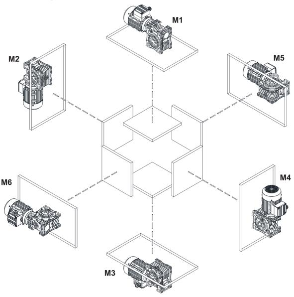
Figured mounting positions of M1 to M6 are determined as reference of directional position of the gearbox. Mounting surfaces are not binding.
