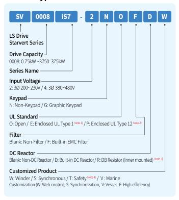
Note 1) For 0.75~75KW range, enclosed type 1 can be satisfied if conduit option installed.
