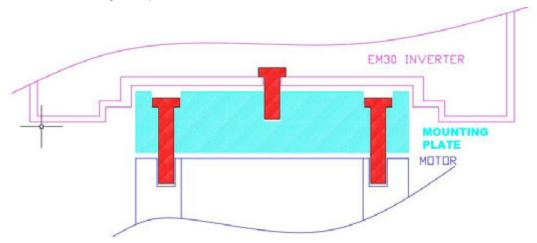
As a first step, the mounting plate must be fixed on the motors terminal box, using original gasket. After the mounting plate is in place, the inverter can be fixed on the plate, using adequate screws and gasket, coming with the plate kit. Specific holes in the capacitor board allow access to the screws inside the inverter. Cabling is done, using the middle hole on the capacitor board
