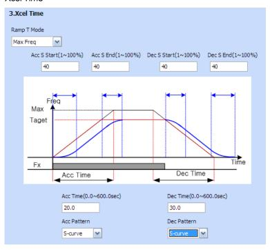
Xcel Time related parameters are output with the graph. The graph changes according to the parameter value selected in the combo. The time range can be changed in the edit window.
