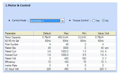
Torque Control is disabled if Control Mode is V/F, V/F PG, or Slip.
