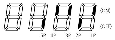
$\times$  Only 1P–3P are available for models equipped with standard I/O.
