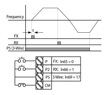
The 3-wire operation latches the signal input (the signal stays on after the button is released) as shown in the diagram above, and is used when operating the inverter with a push button
