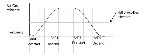
When Acc/Dec reference (bA09) is set to the maximum value while the goal frequency is lower than the maximum frequency, the S-curve is not created properly.
