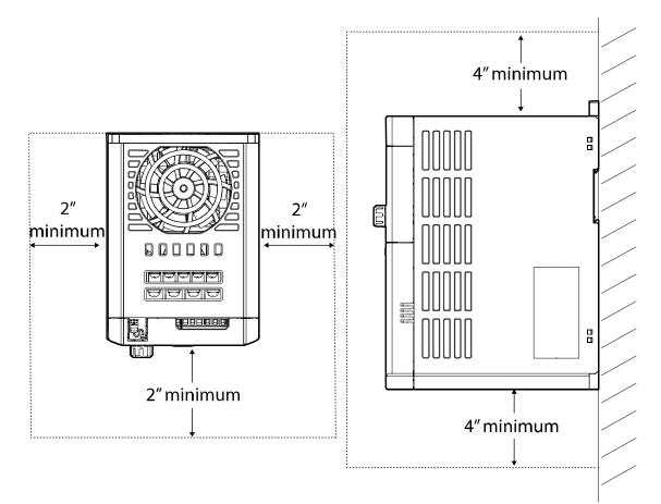
• Ensure sufficient air circulation is provided around the inverter when it is installed. If the inverter is to be installed inside a panel, enclosure, or cabinet rack, carefully consider the position of the inverter's cooling fan and the ventilation louver. The cooling fan must be positioned to efficiently transfer the heat generated by the operation of the inverter.
