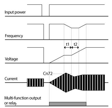
If an instantaneous power interruption occurs and the input power is disconnected, the inverter generates a low voltage trip and blocks the output.
