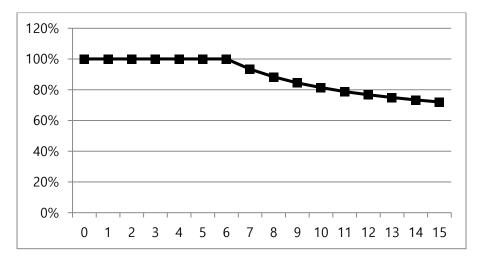
If the ambient temperature is high, and if the maximum carrier frequency for continuous full load conditions (4 kHz for A Frame 0.1 kW-1/0.2 kW-1 products, 6 kHz for B/C Frame 0.4 kW-1 – 2.2 kW-1 products) is exceeded, a protective feature may be activated to limit the carrier frequency (to 4 kHz / 6 kHz) to prevent damages to the product.
