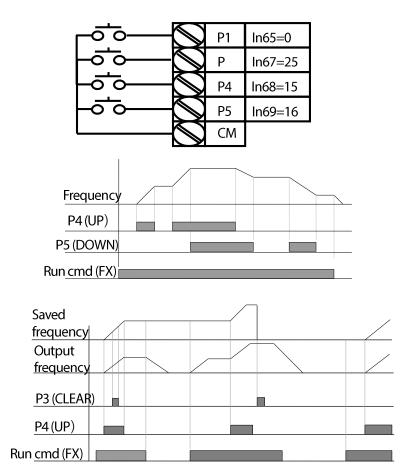
When the Ad66 code is set to 1: The motor accelerates by as much as the step frequency set by the Ad67 code at the multi-function input's positive edge that has been set as the Up terminal signal. The motor decelerates by as much as the step frequency set at the Ad67 code at the multi-function input's positive edge that has been set as the Down signal. The frequency is saved at the falling edge when the Up/down signal is specified. In this case,
