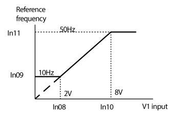
You can connect the terminal wiring as shown below. Refer to the In 07 –11 features.
