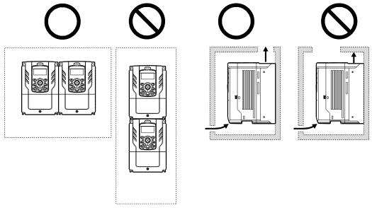
• If you are installing multiple inverters in one location, arrange them side-by-side and remove the vent covers. Use a flat head screwdriver to remove the vent covers. Only the H100 inverters rated for up to 30 kW may be installed side-by-side.
