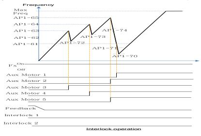
In case that Operable Motor and Standby Motor are set to 3 and 2 each, it operates in the order of "Aux Motor 2  $\leftarrow$   $\rightarrow$  Aux Motor 4  $\leftarrow$   $\rightarrow$  Aux Motor 5".
