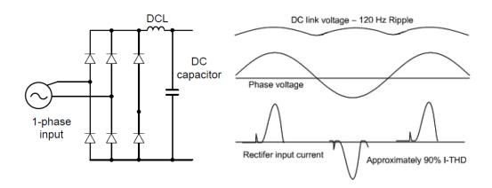
Figure-2 Typical Single-Phase Configuration
