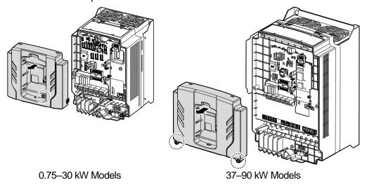
5 Locate the RTC battery holder on the main PCB, and replace the battery.
