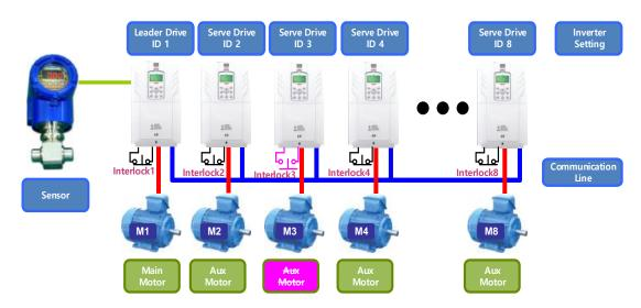
The picture below shows the function in case that M3 becomes HAND/OFF State or interlock and Trip are caused.(supposing that the priority is not changed),(interlock is the function corresponding to B terminal(Normal close)).
