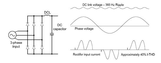
Figure-1 Typical Three-Phase Configuration
