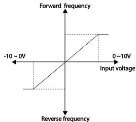
[Bipolar input voltage and output frequency]
