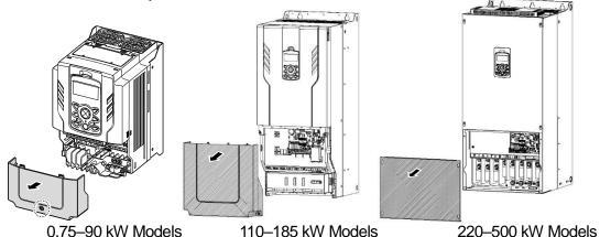
2 Push and hold the levers on both sides of the cable guide (1) and then remove the cable guide by pulling it directly away from the front of the inverter (2). In some models (37~90kW) where the cable guide is secured by a bolt, remove the bolt first.
