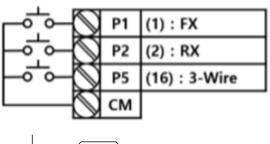
[Terminal connections for 3-wire operation]
