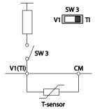
To receive PTC signal at V1 input terminal, set PRT-35 (Thermal InSrc) to '0 (Thermal In)' and set the Analog1 input selection switch (SW3) to T1.
