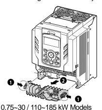
3 Connect the cables to the power terminals and the control terminals. For cable specifications, refer to 1.5 Cable Selection on page 14.
