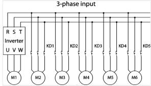
Start order and stop order of the auxiliary motors are based on the order set at AP1-49 (FIFO/FILO).
