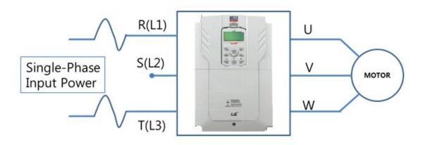
Figure-3 Terminal Wiring Diagram
