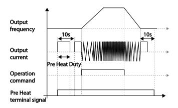
The initial heating operation starts to run after an inverter operation stops, when the initial heating function's terminal input is on after the inverter operation command is off.
