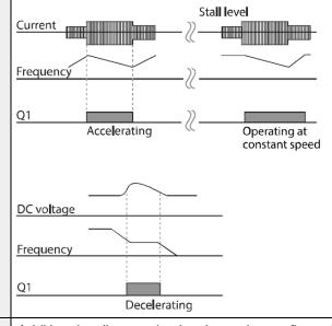
Additional stall protection levels can be configured for different frequencies, based on the load type. As shown in the graph below, the stall level can be set above the base frequency. The lower and upper limits are set using numbers that correspond in ascending order. For example, the range for Stall Frequency 2 (Stall Freq 2) becomes the lower limit for Stall Frequency 1 (Stall Freq 1) and the upper limit for Stall Frequency 3 (Stall Freq 3).
