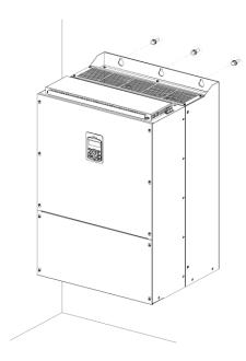
Install the two lower mounting bolts. Ensure that the inverter is placed flat on the mounting surface, and that the installation surface can securely support the weight of the inverter.
