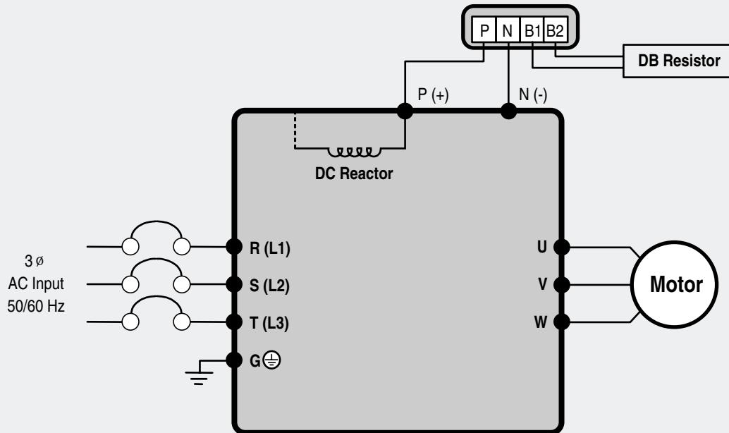
For 37~90kW (50~125HP) Built-in DCL Type
